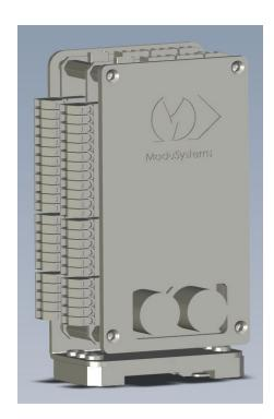
The BLC-2TC is a 4 Axis Modular Controller for controlling 2 Digital Servo Drives or 2 External Stepper Drives.
